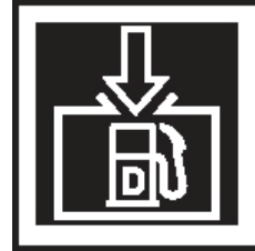
Diesel Fuel Fill
