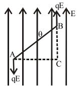
\*\*Note: If the dipole is placed in a uniform electric field, it will experience a torque. Here the net transalatory force acting on the dipole is zero. But if the dipole is placed in a non – uniform electric field, the forces acting on the charges +q and –q will be different. Hence the dipole will experience both translatory force and torque and hence will move sideway in addition to rotational motion.
