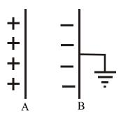
Thus, the resultant force of repulsion on a unit +ve charge is reduced. So the amount of work is less and potential at A decreases. Therefore, capacity of A increases.
