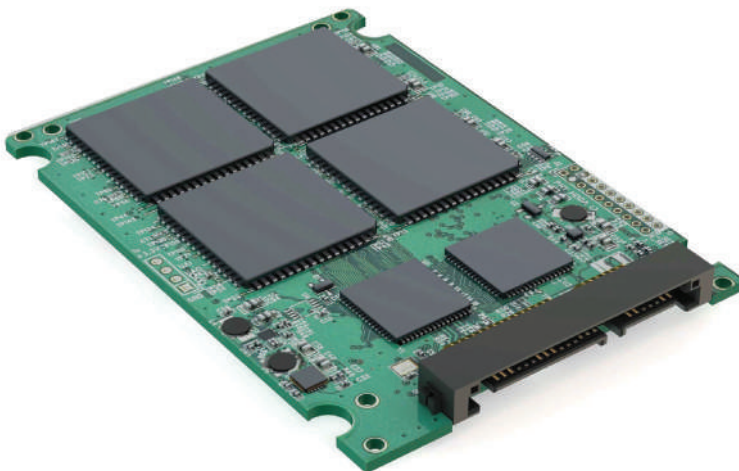
Figure 11.3 A 3.5-inch SSD circuit board.
