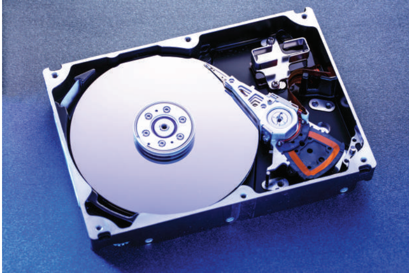
Figure 11.2 A 3.5-inch HDD with cover removed.
