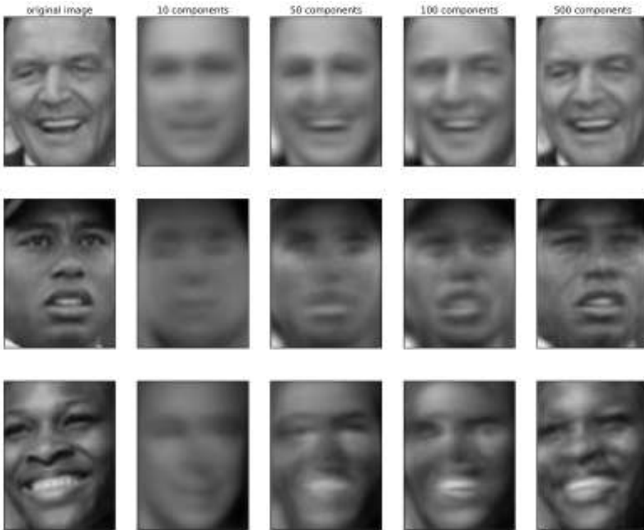
Figure 3-14. Reconstructing three face images using increasing numbers of components found by NMF
