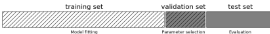
Figure 5-5. A threefold split of data into training set, validation set, and test set
