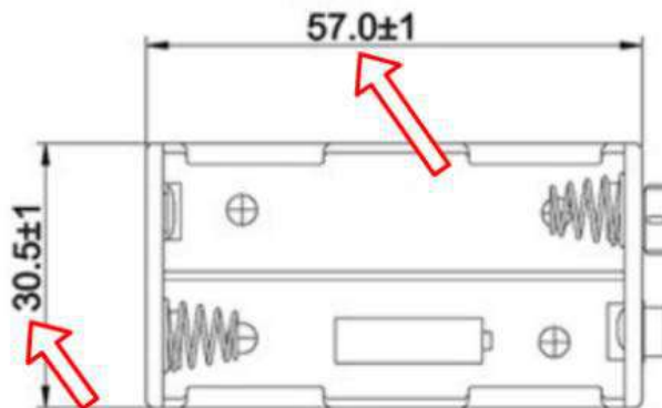
Figure 6.16 – A battery box product drawing with dimensions
