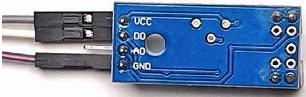
Figure 11.7 – The sensors with cable connections
