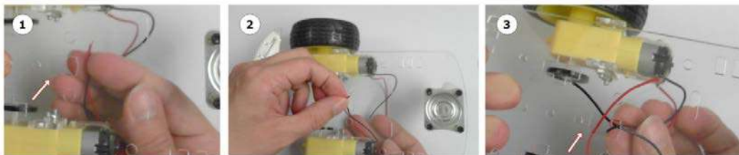
Figure 6.27 – Bringing the wires up
