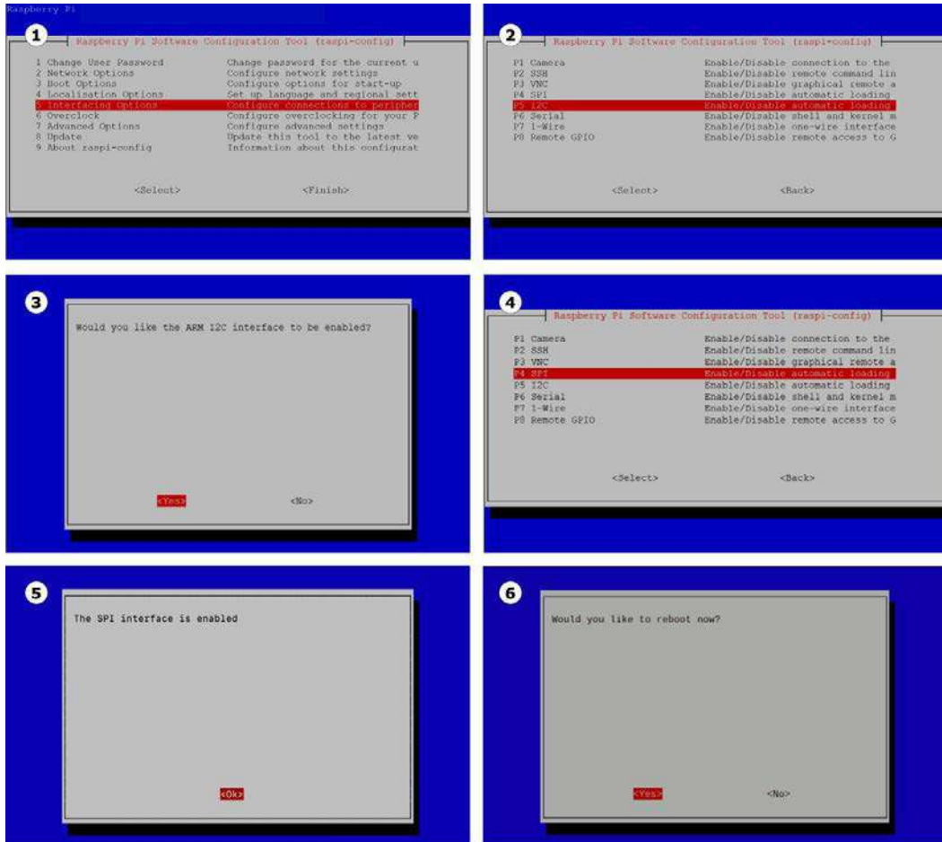
Figure 7.1 – Using raspi-config to enable SPI and I2C
