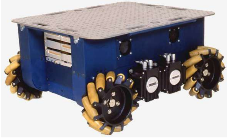
Figure 7.5 – Mecanum wheels on the Uranus Pod by Gwpcmu [CC BY 3.0 ( https://creativecommons.org/licenses/by/3.0 )]
