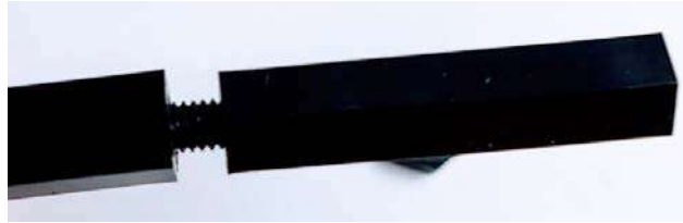
Figure 12.6 – Joining the standoff posts
